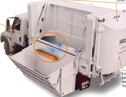
Unique panel design facilitates material flow during the compaction cycle to achieve higher payloads.
